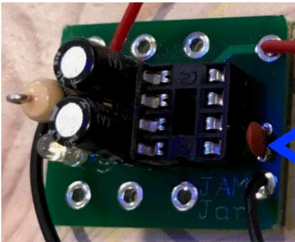
For those who have the old style board the capacitor needs to be soldered across pins 1 on the chip socket and negative output.
